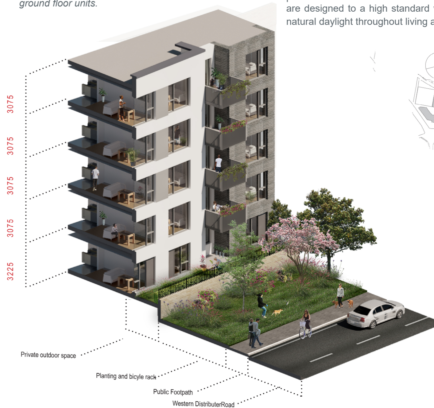
Sectional Elevation along Gort Na Bro / Western Distributer Road road showing separation of public and private realm
